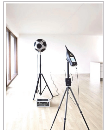
Sound Insulation Testing On-site
